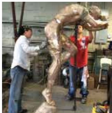
METAL CHASED: Marcus and the fabricators use precision tools to chase the raw metal, which means refining it, disguising its joints, and restoring its texture.
