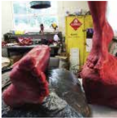
WAX REWORKED: The rubber mold is moved to the foundry, where wax is poured into it. Marcus then reworks the dried wax form. Here her reworked wax awaits "gating," during which wax sprues will be attached so that molten bronze will flow evenly later in the process.
