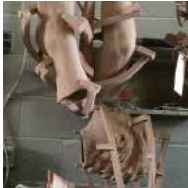
WAX DIPPED: One by one, sections of the wax form are dipped in a slurry mixture of silica and mulgrain to encase them in a thick ceramic shell. This is repeated 12 times and requires drying between each dip. Once placed in the hot kiln, the wax "burns out" to leave behind a hard ceramic, thus the term "lost wax method."
